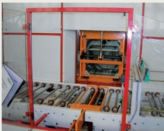
The glass doors allow the cleaning and drying processes to be carefully monitored and adjusted.
