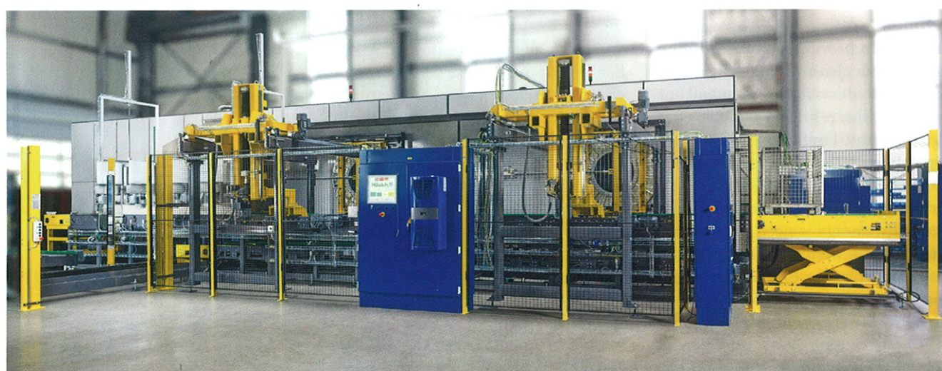
Front view of the two-chamber cleaning and degreasing machine with part of the transport system.
