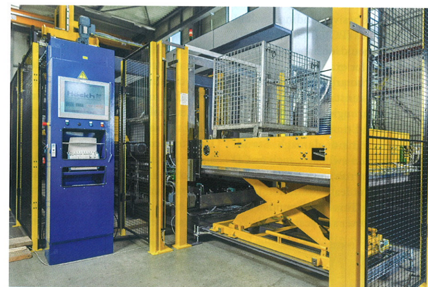
The wire mesh pallets are loaded onto the machine using forklift trucks. Large graphical control and display panels make the complex machine easy to use and to monitor.
